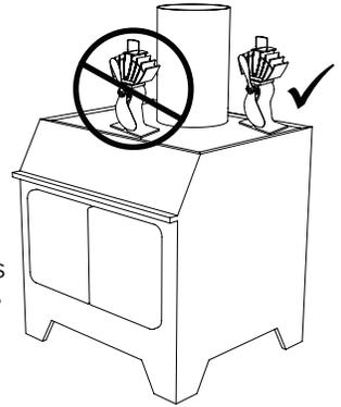
NOTE: Overheating will reduce the Ecofan's effectiveness and may damage the thermoelectric module and void the warranty. Remove the Ecofan from stove if temperature exceeds 650°F (345°C).
